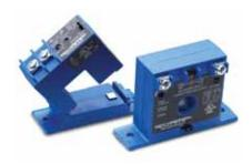
ACS200 series current operated switches provide the same dependable status indication as the ACS150 series, but with added resolution. A choice of three jumper-selectable input ranges allows the ACS200 to be tailored to an application and provides more precision in setpoint adjustment. Self-powered, isolated solid-state relay outputs and multiple input ranges are standard features.
