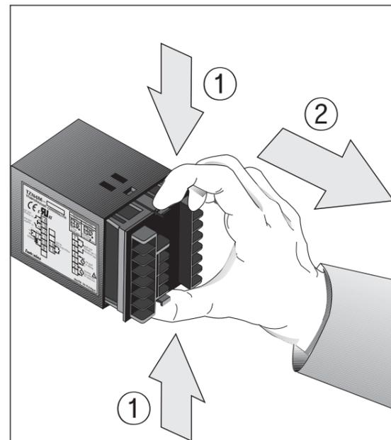
\*Case detachment : Pull the handle backward after press both side of it on terminal block.
