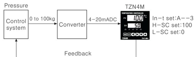
\*In case of using the converter mode, please select the inner switching pin according to the chart in "Selection switch for Input sensor/Voltage/Current".
