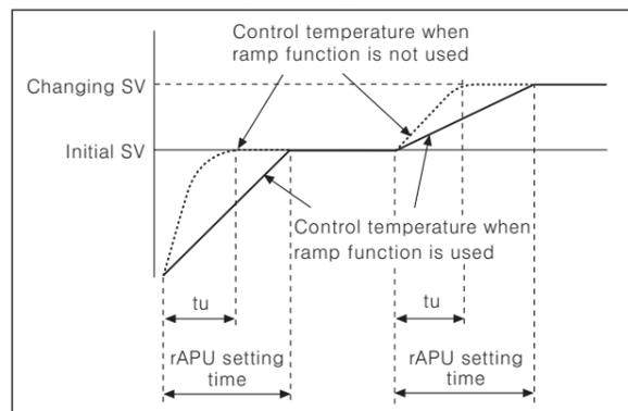
It makes delay rising temperature when change the set value at stable control status or delay the initial rising temperature as above picture. Note1)rAPu time cannot be set shorter than temperature rising time(tu), when Ramp function is not used.
