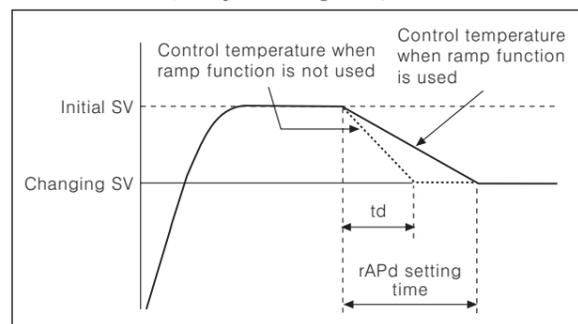
It controls falling temperature as above. Note1)rAPd time cannot be shorter than falling time(td) of not being ramp function operated.
