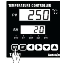
4 Press **MD** key when the setting is completed. It will stop flickering, then return to RUN mode.
