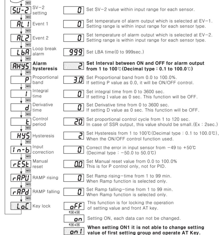
\*It will start to flicker by pressing **Key** and the flicker will be moved by **Key**, **Key** keys then set the value by **Key**, **Key** keys. After that if pressing **MD** key the DATA will be changed then display next mode.
