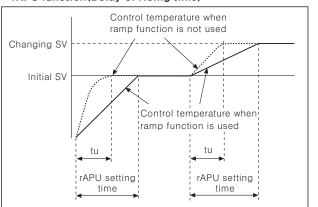
It makes delay rising temperature when change the set value at stable control status or delay the initial rising temperature as above picture.
