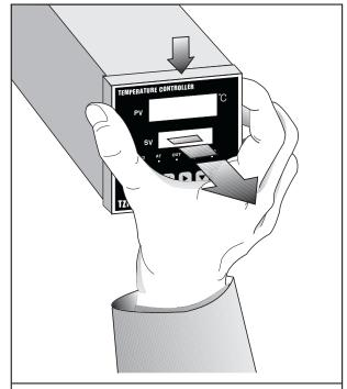
\*How to take out the inner body from the case: Pull the front panel guide to forward on pushing it to down direction.
